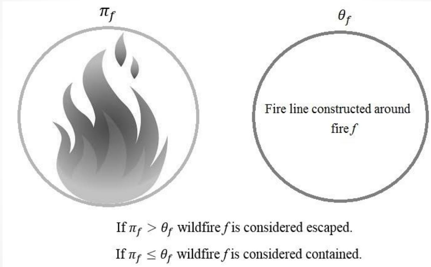
**Fig. 2.** Containment condition
